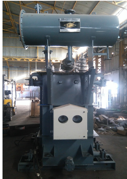
EHV Transformer of 5 mVA Capacity
